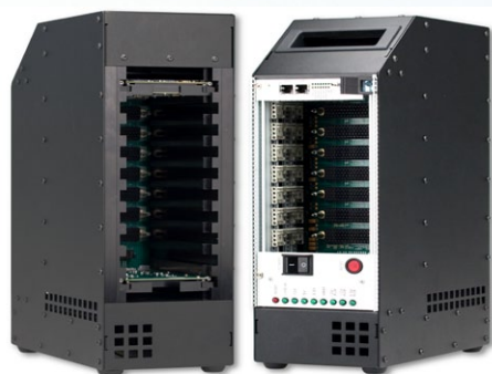
XPand1200 3U VPX Development Platform for Conduction-Cooled Modules
