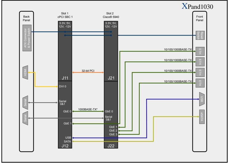
\*Connection between slots made via bottom-side cat5 jumper cable which can be removed for custom configurations, allowing direct access to SBC GbE0 and Cisco 5940 GbE0 ports
