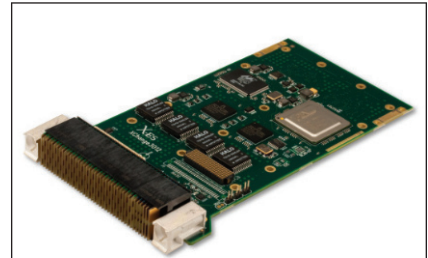
Figure 2 | The Extreme Engineering Solutions (X-ES) XChange3012 OpenVPX 3U integrated switch
