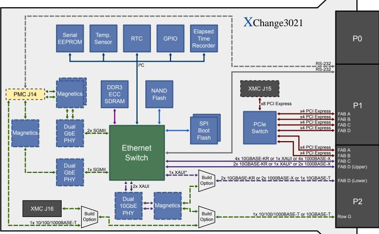
Dotted lines indicate optional functionality that is not supported on all configurations. Contact X-ES Sales for more information. \* Both FAB D (Upper) and FAB D (Lower) must be configured for XAUI to support the 1x XAUI link.
