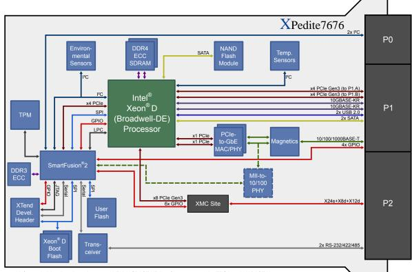
\*A factory build option allows the second VPX 10GBASE-KR interface to route to the FPGA as 1000BASE-X. This option will reduce the SmartFusion<sup>®</sup>2 PCI Express interface to x2.
